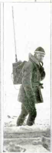
Broadcasting from a bobsled skimming over ice at 70 miles per hour! The transmitter is strapped to No. 3 man. A 5 ft. vertical rod is the antenna. A close-up of the 7-meter, 1-watt transmitter is shown (right) on the operator's back.
