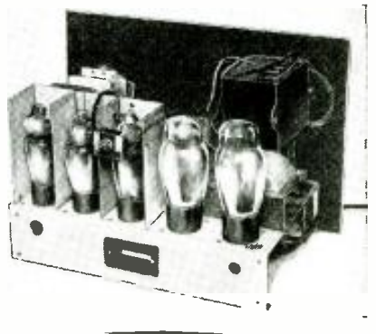
Fig. B, below The radio receiver portion of the system.
