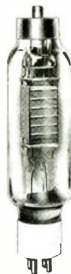
Fig. 1 The internal appearance of the RK-31 showing how the two grids are connected together.
